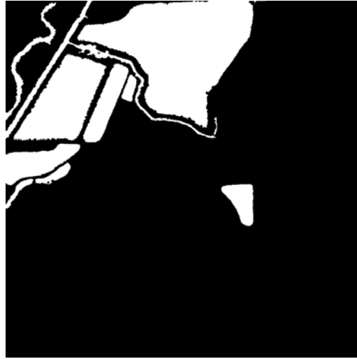
Figure 10. Water body detected after merging detection from method 1 and method 2
