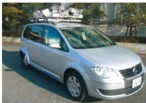
Figure 1. Appearance and size of Mobile Mapping System (Mitsubishi Electric Corporation, 2012)
