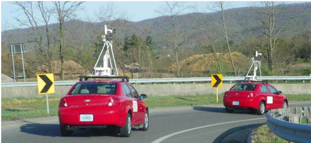
Figure 2. Two of the mobile mesonet units, mounted on Chevrolet Cobalts, driving off I-81 into Roanoke, Virginia on April 21, 2013
