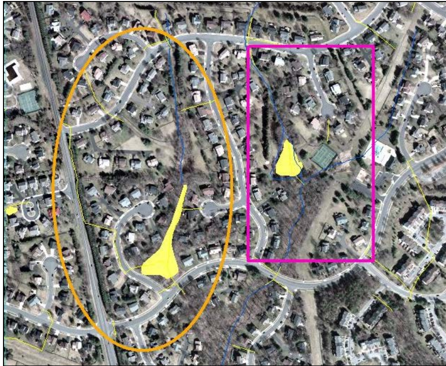
Figure 6. Isolated storm networks and retention ponds (orange oval), a stream channel and storm pipes (yellow lines) that direct water flow into a storm retention pond. An area where storm drain pipes actually connected disconnected stream channels to the main stream channel (fuchsia rectangle).
