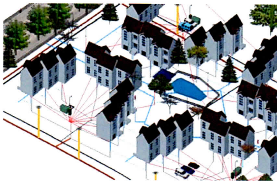
Figure 7. Photo-realistic view of the townhome complex with underground power lines (from each transformer) (in red), sewer lines (in brown) and water lines (in blue)
