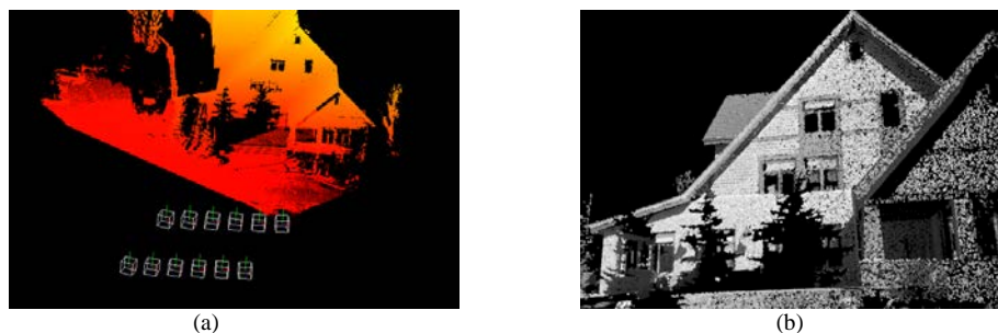
Figure 7. (a) 12 virtual cameras are placed in front of the Ronald McDonald House; (b) one intensity image generated from the point cloud acquired by Faro Focus 3D laser scanner
