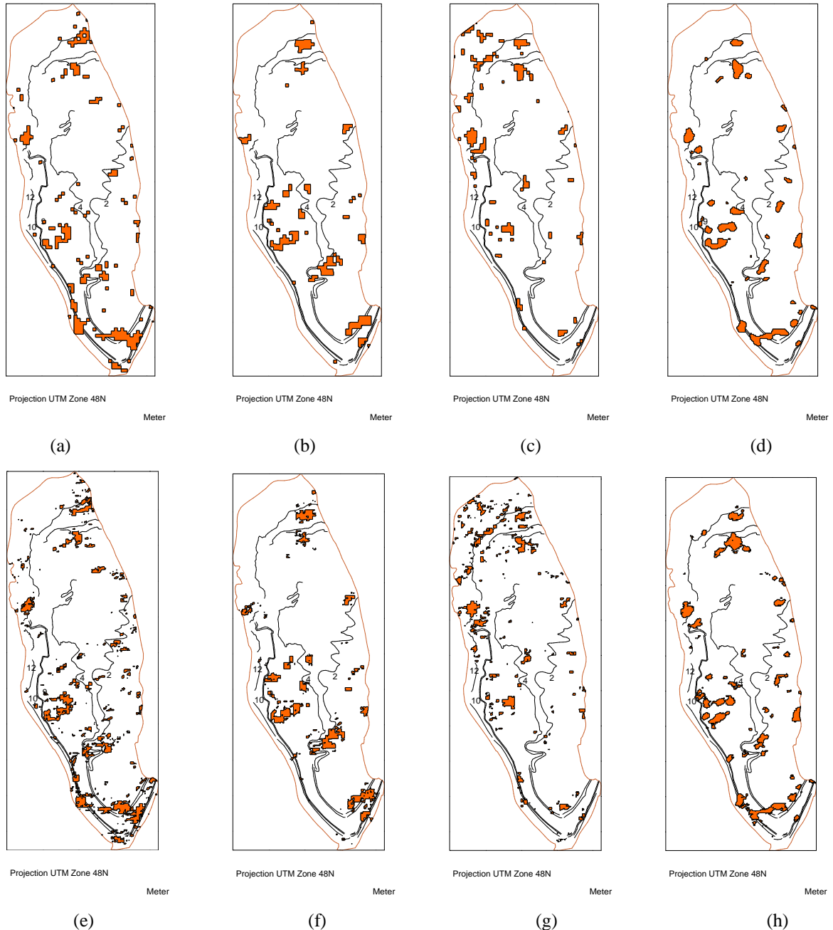
Figure 5. Thermal anomalies from original thermal infrared images and from solar radiation corrected images for four typical seasons: March. 27 2013, June 22 2013, September 26, 2013 and December 23 2013 were mapped, listed as follows. Coal fires from original TIR images for: (a) 2013/03/27; (b) 2013/06/22; (c) 2013/ 09/26; (d) 2013/12/23; Coal fires from solar radiation corrected images for: (e) 2013/ 03/27; (f) 2013/ 06/22; (g) 2013/09/26;
